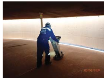
Fig.40 Tank floor scan by magnetic flux leakage on bottom plate.
