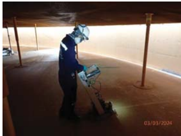
Fig.37 Tank floor scan by magnetic flux leakage on bottom plate.
