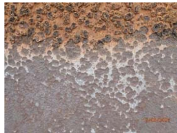
Fig.16 Corrosion on internal shell 0.5-2 mm depth (shell course 2).
