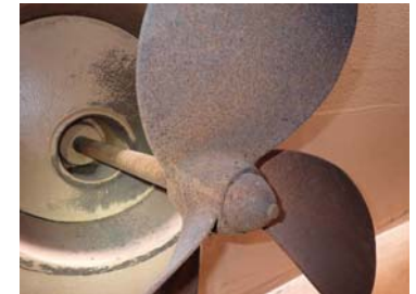
Fig.26 Surface corrosion on mixer.
