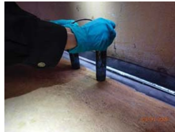
Fig.46 Magnetic particle examination on shell-to-bottom welds
