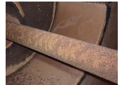
Fig.28 Surface corrosion on mixer.
