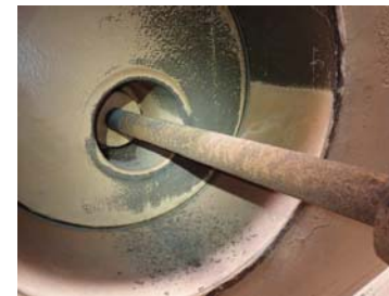
Fig.27 Surface corrosion on mixer.
