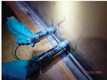
Fig.45 Magnetic particle examination on shell-to-bottom welds.
