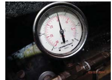
Fig.44 Vacuum box test on shell-to-bottom welds.
