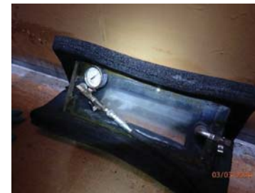
Fig.43 Vacuum box test on shell-to-bottom welds.
