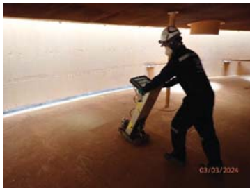
Fig.39 Tank floor scan by magnetic flux leakage on bottom plate.
