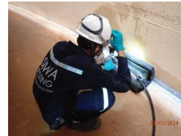
Fig.41 Vacuum box test on shell-to-bottom welds.
