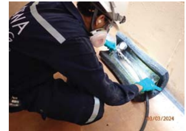
Fig.42 Vacuum box test on shell-to-bottom welds.
