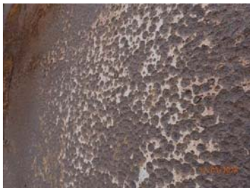
Fig.15 Corrosion on internal shell 0.5-2 mm depth (shell course 2).
