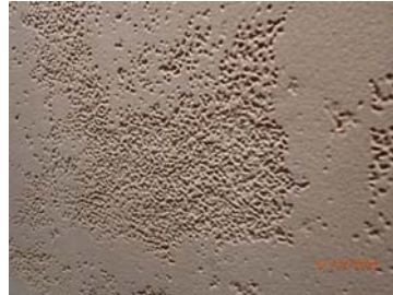
Fig.14 Corrosion on internal shell 0.5-2 mm depth (shell course 1).
