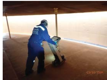
Fig.38 Tank floor scan by magnetic flux leakage on bottom plate.
